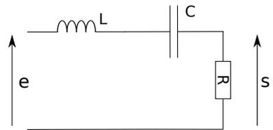
$\underline{H}(j\omega) = \frac{jRC\omega}{1 + jRC\omega - LC\omega^2}$ | <p>Montage RLC coupe-bande</p>
