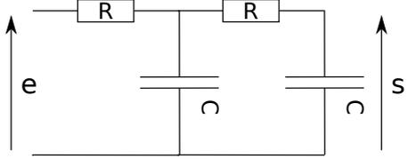
$\underline{H}(j\omega) = \frac{1}{1 + 3jRC\omega - (RC\omega)^2}$                   | <p>Montage double passe-haut</p>
