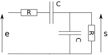
$\underline{H}(j\omega) = \frac{jRC\omega}{1 + 3jRC\omega - (RC\omega)^2}$ | <p>Montage coupe-bande</p>
