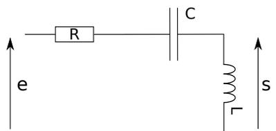
$\underline{H}(j\omega) = \frac{-LC\omega^2}{1 + jRC\omega - LC\omega^2}$     |
