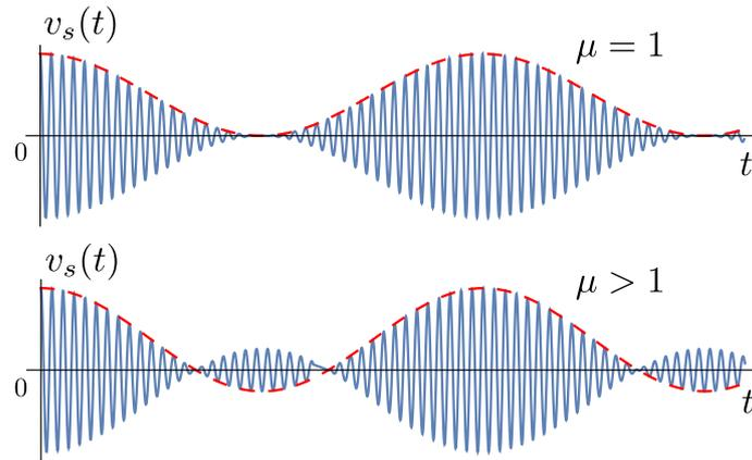
FIGURE 63 – Cas  $\mu = 1$  (haut) et  $\mu > 1$  (bas).
