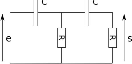
$\underline{H}(j\omega) = \frac{-(RC\omega)^2}{1 + 3jRC\omega - (RC\omega)^2}$           |
