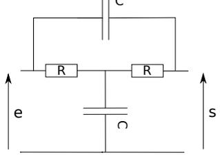
$\underline{H}(j\omega) = \frac{1 + 2jRC\omega - (RC\omega)^2}{1 + 3jRC\omega - (RC\omega)^2}$ |
