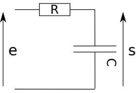
$\underline{H}(j\omega) = \frac{1}{1 + jRC\omega}$ | <p>Montage passe-haut (pseudo-dérivateur)</p>
