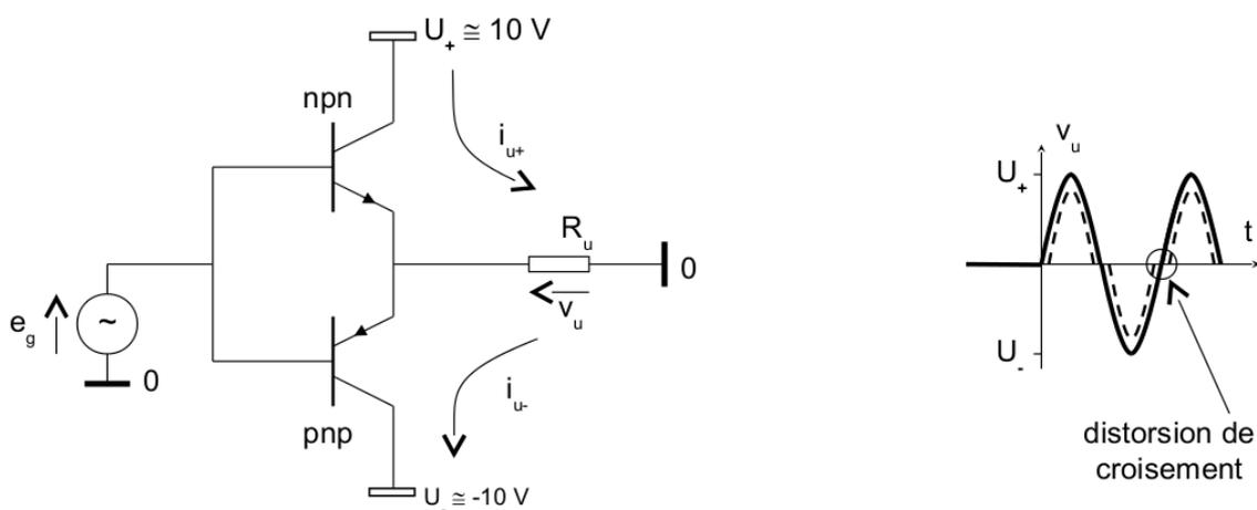
FIGURE 111 – Montage Push-Pull.
